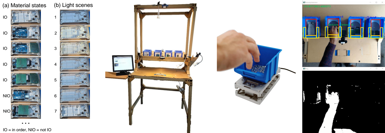
Fig. 3 Assembly workstation equipped with 1 touch screen, 2 cameras and 6 light sources (middle); example material states (of the 38) and 7 light scenes for one part (left); inventory control with weighting pad, and grasp detection using background subtraction with the ‘U’-shaped activity zones (right).
