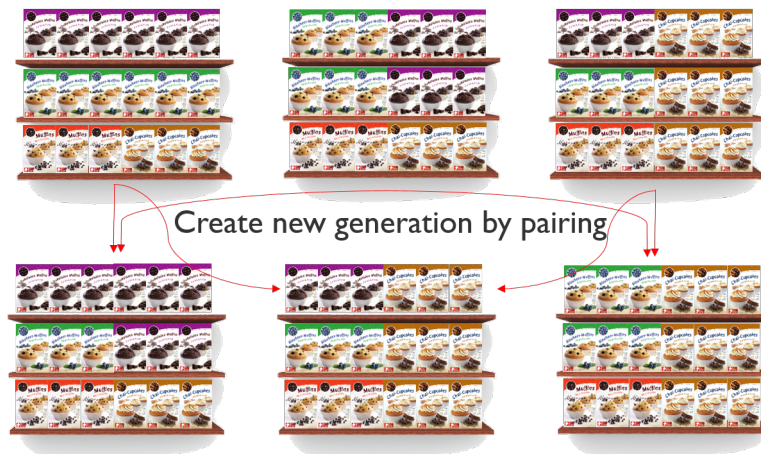
Figure 2.3: Crossover in the genetic algorithm by concatenating left and right halves of the parent shelves.
