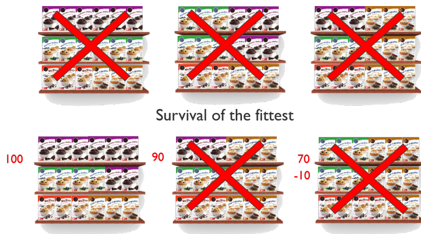
Figure 2.7: Survival of the fittest in the genetic algorithm: bad solutions are removed with high probability.
