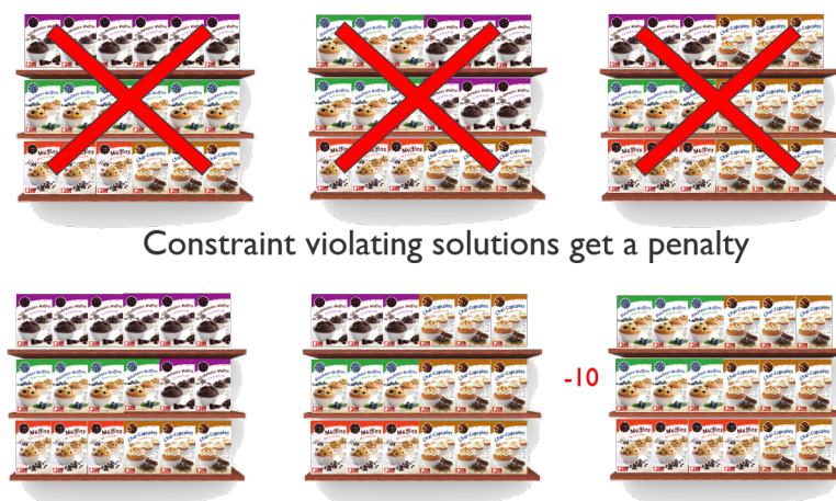
Figure 2.6: Constraint violating solutions get a penalty in the genetic algorithm. Assume for example the maximum facing amount of the red product is three.
