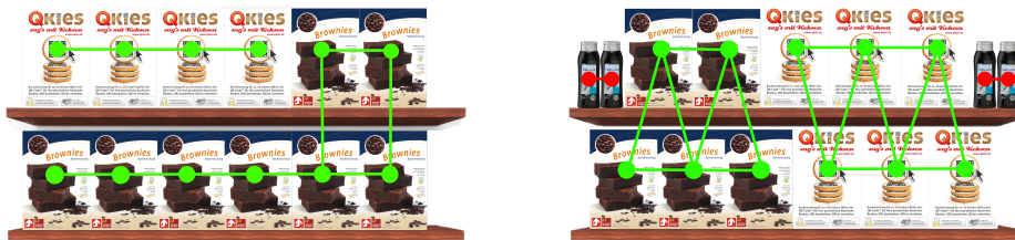
Figure 4.8: The left picture shows the graph of a valid solution as all product instances are connected, while the right image shows the graph upon a more complex and forbidden placement where products are arranged in an offset pattern.
